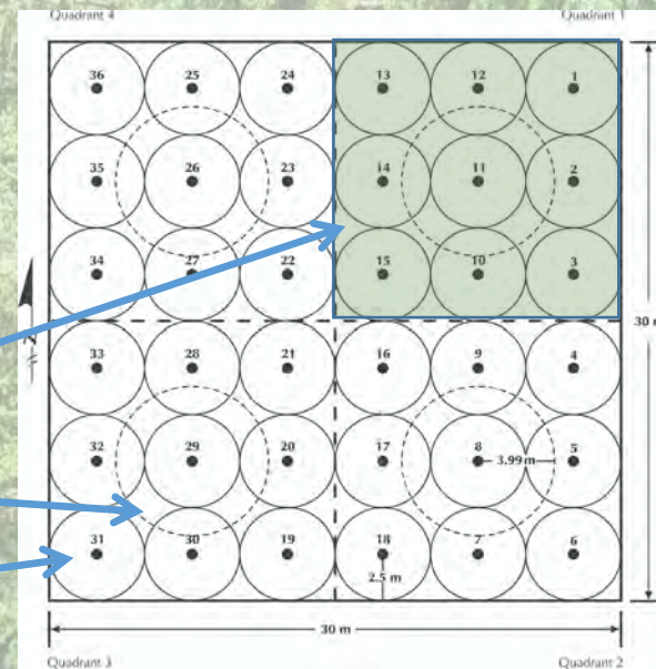
Figure 2. Layout of a measurement plot using the TRENDS © silvicultural protocol illustrating quadrants, 3.99 m radius subplots, grid points and numbering convention.
